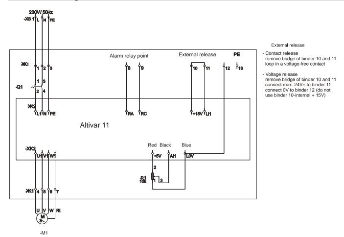
The control binders that are not connected provide for a number of additional functions and monitorings, which are to be selected through parameterization. A detailed description can be found in the operating instructions of the frequency converter.
