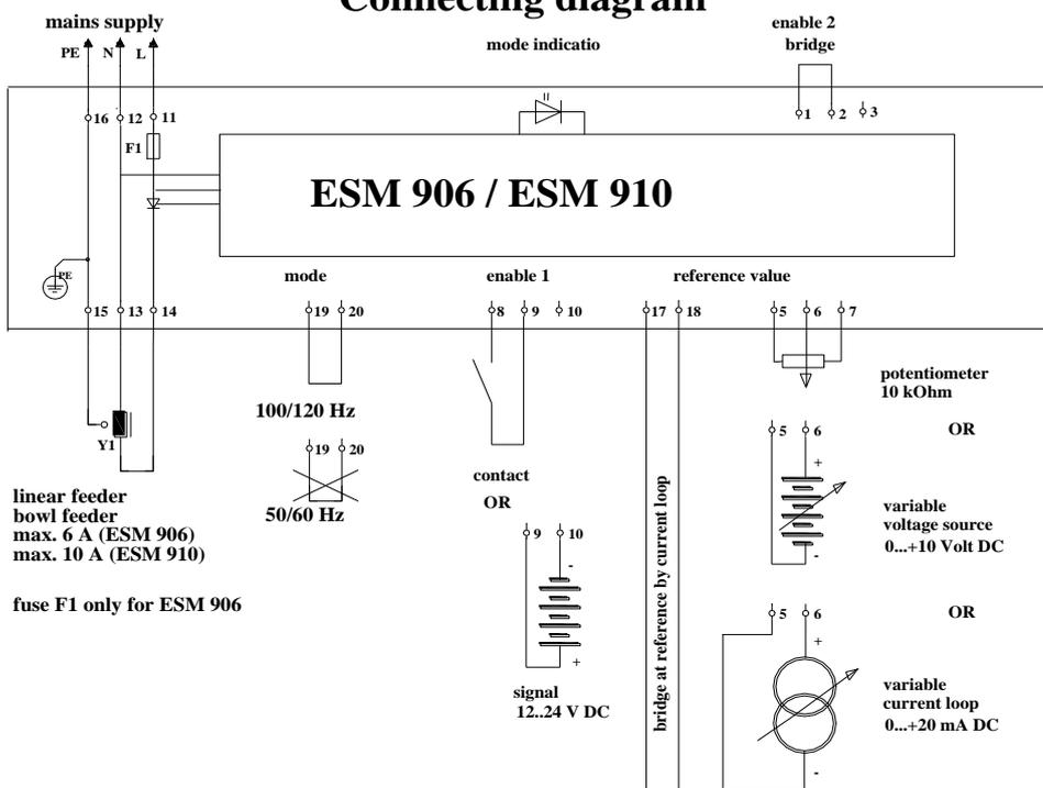
Note: The connecting diagram for the Modul ESM910 is identical. Only the two statusoutputs on clamp 1 upto 4 are not available. Here the clamp 1 and 2 have to bridge.
